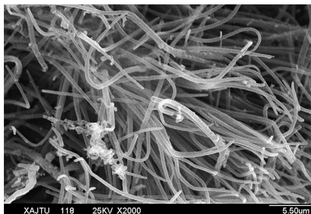
Fig. 6. SEM image of cylindrical PPY micro/nanotubes (pyrrole: 0.31 \text{ mol L}^{-1} , Acid Red 1: 0.062 \text{ mol L}^{-1} , \text{FeCl}_3 : 0.52 \text{ mol L}^{-1} , 278 K, stirring rate \geq 200 \text{ rpm} ).
